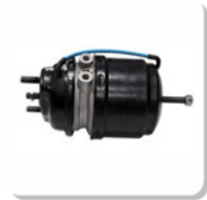
CILINDRO TRISTOP BAIONETA TRISTOP BRAKE CHAMBER
