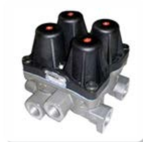
VALV. PROT. 4 CIRCUITO 4 WAYS PROTECTION VALVE
