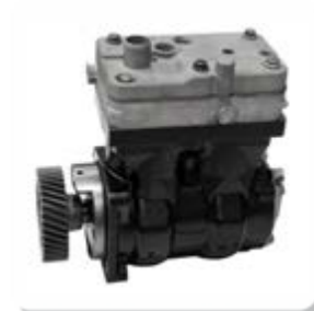
COMPRESSOR AR AIR COMPRESSOR KNORR TYPE
