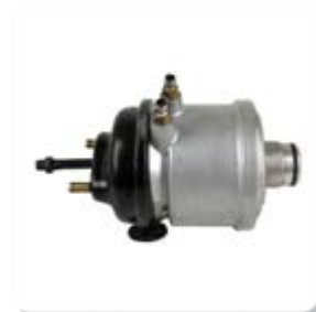
CAMARA SPRING BRAKE 30 BRAKE CHAMBER 30
